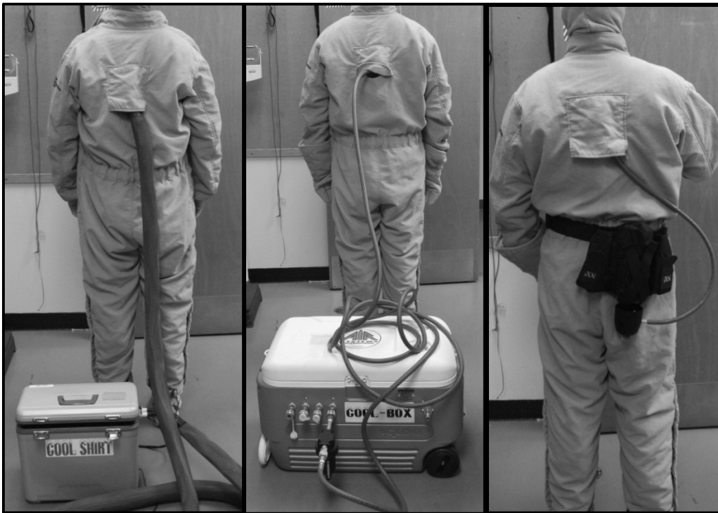
Figure 3. Pictured from left to right: 1) CoolShirt ® Aqua Vest system, 2) Allegro ® air vest with Cool-Box air cooling system (Air Systems Inc.), and 3) Porticool II ® cooling system secured to the participant with a paintball bottle belt (NX e ®). Each cooling vest was worn under the Gas Extraction Suit ® and Nomex ® coverall and over a T-shirt.
